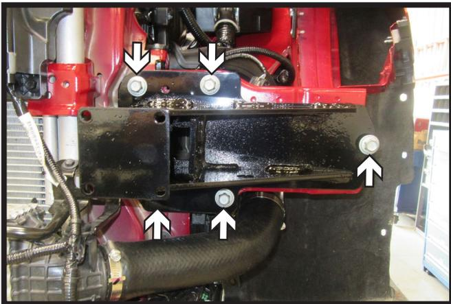
15. Hold the side plate in place and start the five (5) existing 14MM bolts. Do this on both sides of the vehicle.
