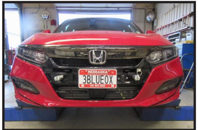
20. Reinstall the air baffle. Hold the fascia as close to its original position, mark and trim the fascia around the convenience links and attachment tabs. Reinstall the belly pan, headlights, fascia and fascia cover. Reconnect all electrical connections.
