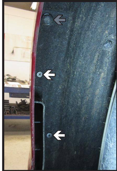
3. Using a Phillips screwdriver, remove the two (2) screws (white) from the wheel well. Then remove the one (1) push pin (gray). Do this on both sides of the vehicle.
