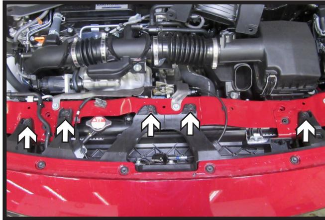
6. Using a 10MM socket, remove the five (5) bolts along the top of the vehicle.
