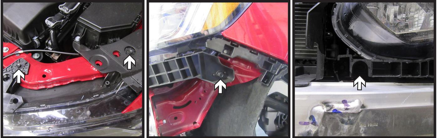
7. Using a 10MM socket, remove the four (4) bolts from the headlight. Remove the headlight and set aside to be reinstalled later. Do this on both sides of the vehicle.
