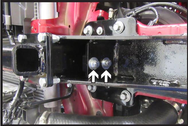
17. Slide mounting strap into place and start two (2) 3/8" x 1-1/4" bolts with flat washer and lock washer, leave loose. Do this on both sides of the vehicle.
