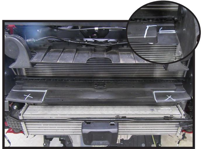
14. Using a utility knife trim both sides of the air dam as shown. Make sure to trim the extra area on the driver side of the vehicle (inset) to allow room for breakaway bracket.
