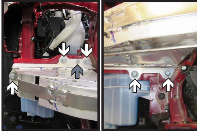
8. Using a 14MM socket, remove the five (5) bolts (white) from the bumper. Then using a 10MM socket, remove the one (1) bolt (gray) from the top of the bumper. Do this on both sides of the bumper. Remove bumper, it will not be reinstalled later.
