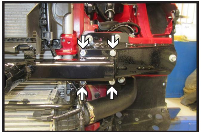
16. Attach the cross tube to the side plates using eight (8) 3/8" x 1-1/4" bolts with nylon lock nuts, there are four (4) bolts on each side of the vehicle. Remove each side plate bolt, apply Loctite® Red, and reinstall. Tighten fully.
