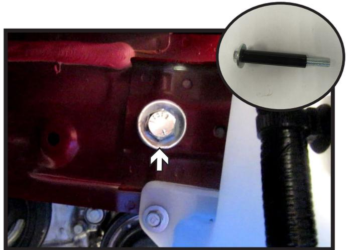
18. Place spacer tube on 1/2" x 4-1/2" bolt with flat washer (inset) and install bolt with second flat washer and nylon lock nut into back frame hole. Do this on both sides of the vehicle. Tighten front mounting strap bolts fully at this time.
