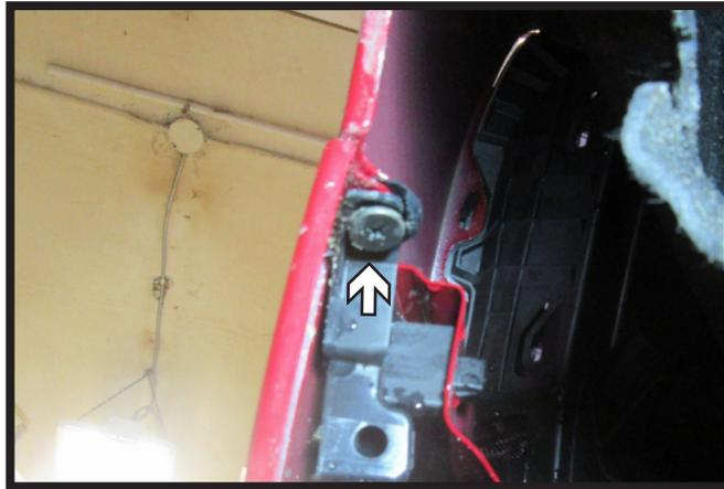
4. Pull back the wheel well liner and using a Phillips screwdriver, remove the one (1) screw. Do this on both sides of the vehicle.
