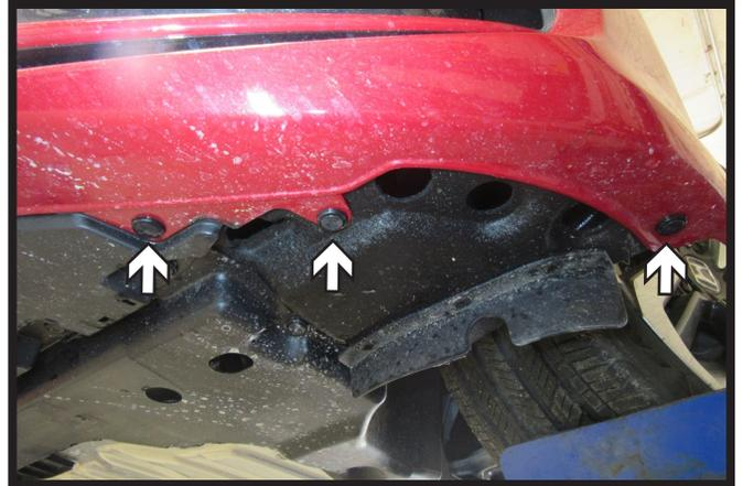
5. Remove the twelve (12) push pins from the underside of the vehicle, there are six (6) on each side. Remove fascia and unplug any electrical connections, set aside to be reinstalled later.
